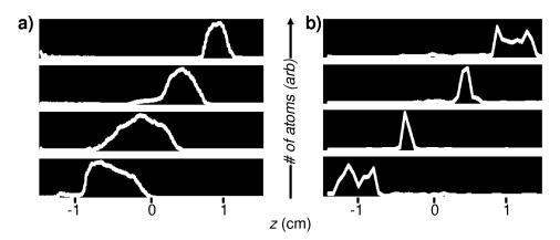
Fig. 3. The effect of the cooling beam intensity imbalance on trap formation. a1)-a4) Experimental longitudinal atomic density profiles that result when  $\theta = 0$ , OD= 10,  $\delta = -1.5\Gamma$ ,  $I_c^+:I_c^-= 25:4$ , 5:3, 3:5, 4:25. b1)-b4) The result of numerical simulations modeling the effects of intensity imbalance when  $\theta = 0$ , OD= 10,  $\delta = -\Gamma$ ,  $I^+:I^-= 3:2$ , 5:4, 4:5, 2:3 (note that OD here is defined for unsaturated absorption).
