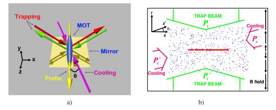
Fig. 2. a) The experimental beam geometry. The trapping beams are in the x - y-plane oriented at 45° to the *y*-axis and the cooling beams are in the x - z-plane. b) The model beam geometry with effective cooling and trapping beams shown. Also, the relative direction and magnitude of the magnetic field are shown.
