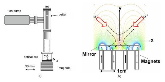
Fig. 1. a) The atom trap setup. b) Magnetic field contours (0.6 G/line) resulting from the magnetic cores (only a portion of the cores is shown). The orientation and polarization of the trapping beams (red arrows) are also shown, along with the orientation of the quadrupolar field lines.
