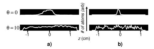
Fig. 4. a) Experimental longitudinal atomic density profiles of traps obtained for equal intensity cooling beams at  $\theta = 0^{\circ}$  and  $10^{\circ}$ . b) Numerically modeled atomic density profiles for equal intensity cooling beams at  $\theta = 0^{\circ}$  and  $10^{\circ}$ .
